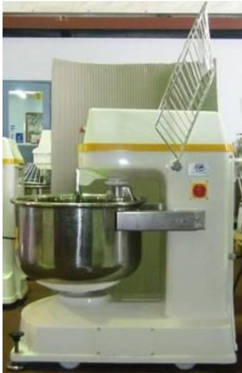
Fig1.7 Safety guard in raised position
